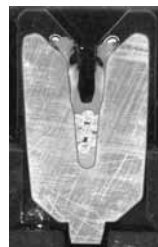
Cross section of wire crimped in the lower tier
